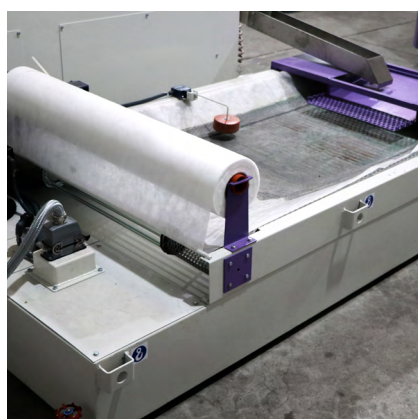
__ AWF200 automatic filtration system in an independent unit
