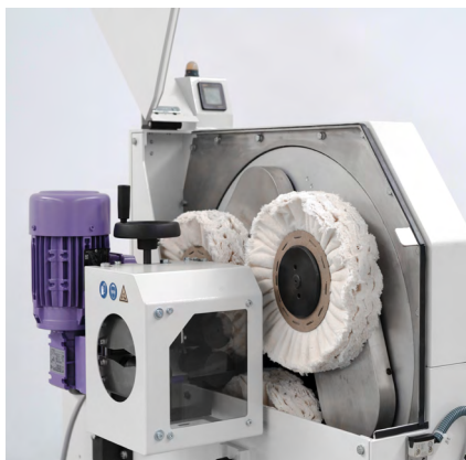
__ planetary polishing system that consists on three planetary polishing wheels wich rotate around the tube applying high pressure
