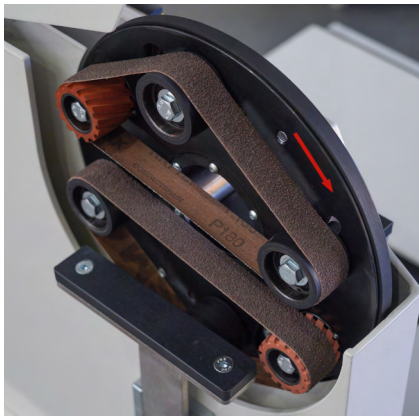
__ slim and compact planetary wheel with 2 abrasive belts
