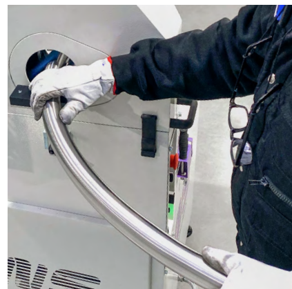
easily removable feeding units for bent tube finishing
