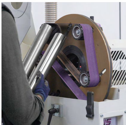
planetary wheel with 2 abrasive belts
